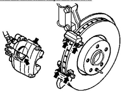
Clean and check brake pad mating surfaces in the brake caliper and caliper holder. Check piston dust boot. Replace dust boot if it is damaged.
