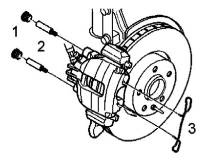
Lubricate the locating pins (2) with grease, P/N 1161325-4. Insert the locating pins into the rubber sleeves. The pins should slide into the sleeves easily. Tighten locating pins. Tighten to  $\bf 30~Nm$ . Install protective caps (1). Install the retaining spring (3).
