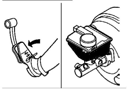
Depress the brake pedal a few times. Check the level of the brake fluid reservoir. Top up if necessary.
