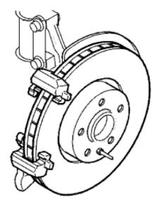
Check brake disc friction surfaces.
