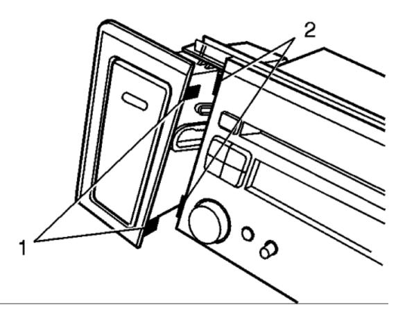
\* Press the mug holder into place beside the radio. Ensure that the mug holder catches (1) engage in the corresponding hooks (2) on the radio.
